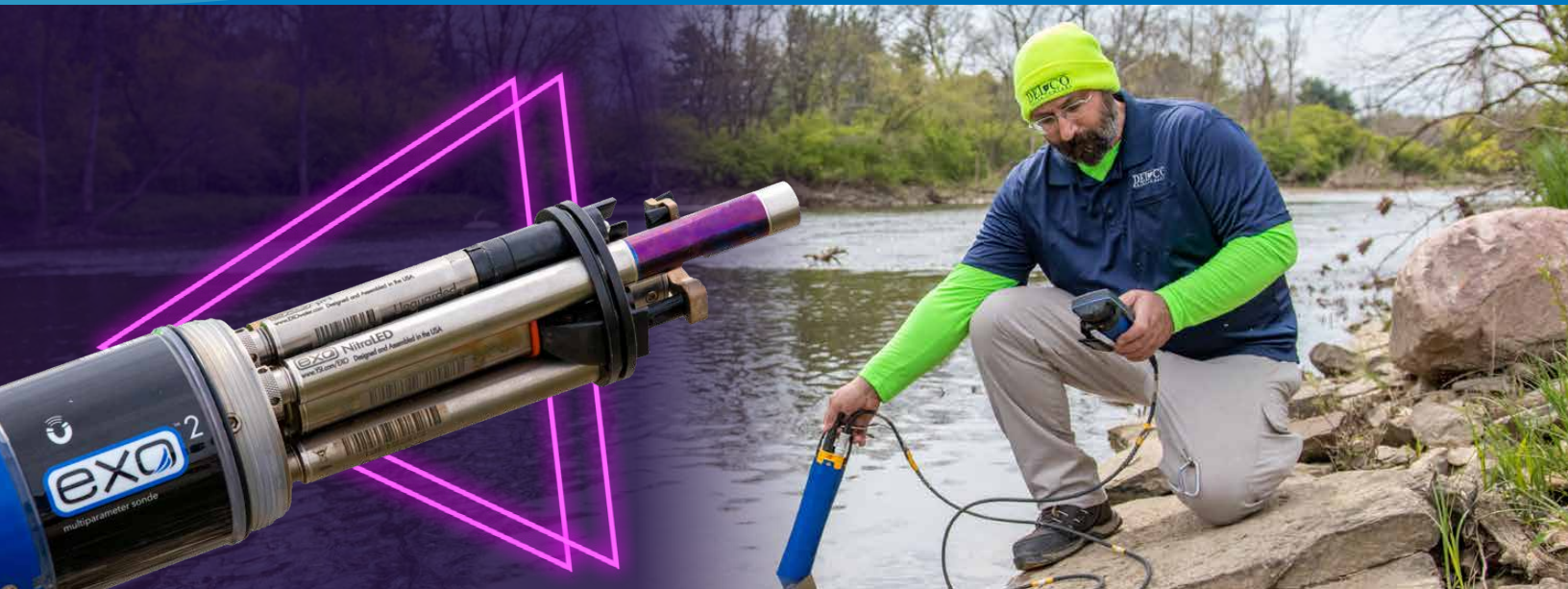
Fred Milan of Del-Co Water uses the NitraLED UV Nitrate Sensor on an EXO Sonde to monitor water quality in drinking water reservoirs.
